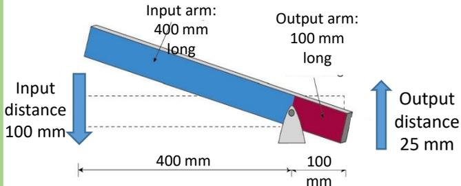
**Output ÷ Input x Input distance = Output distance**
