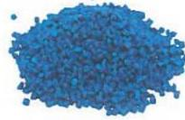
Powders and granules are mainly used in plastic processing such as plastic dip coating, injection moulding and extrusion. The granules are heated until they become soft and can then be shaped as required. Powders tend to be bonded to the surface of hot materials such as metals. Both are available in a wide range of colours.
