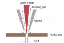
Laser cutters are one of the most accurate ways to cut a number of different plastics. (Note that use of some plastics, for example PVC, should be avoided as they will give off poisonous fumes when heated.) The laser itself can follow a design to a very fine tolerance, but they must be set up correctly considering the following.
