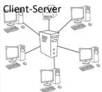
The network relies on a central server and all the clients (devices) request services from the server such as print services, file services etc. Additional hardware is needed in this type of network: a server. All files can be stored and backed-up centrally on a server which means workers can access files from any computer on the network and the computers can also be updated centrally.
