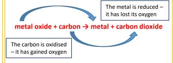
This works for **zinc**, **iron**, **tin**, **lead** and **copper** because they <u>all less reactive</u> than carbon.
